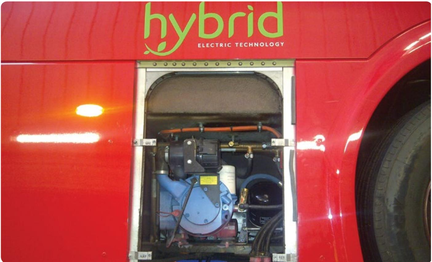
Compressor running is matched to meet the changing demand for air. Inverter drive technology controls the speed of the compressor to provide the amount of air required by the vehicle systems at all times.
