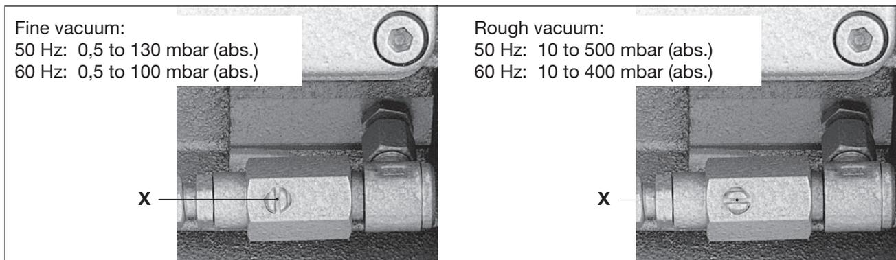
Fig. 4 Version (09): Setting the operating range
