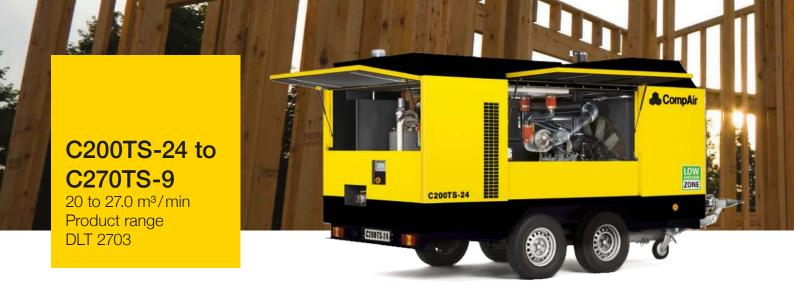
The TurboScrew compressors with their unique patented bi-turbo technology provide class-leading diesel efficiency, the lowest weight of 3,500kg and super-clean performance in accordance with directive 97/68/EC Stage V. The new range has been equipped with an award winning SCRT® – Selective Catalytic Reduction Technology system which is capable of removing almost all nitrogen oxide emissions from diesel exhaust gases.
